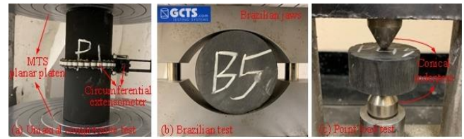
Fig. 13 Loading conditions of UCS test, Brazilian test, and PLT
