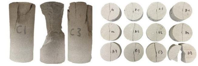
(a) Uniaxial compressive test (b) Point load test
